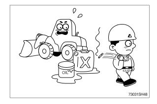
Spilled grease and oil are dangerous to safety. Keep your machine always clean and dry.
